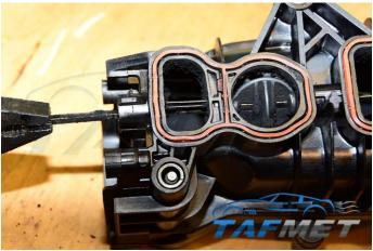
Using pliers to hold the swirl flaps rod, pull and remove the rod.
