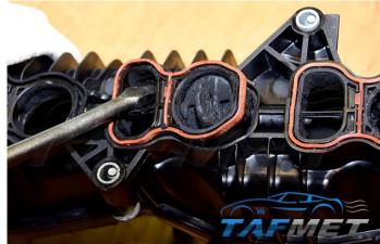
Pull the sockets, in which the swirl flaps are hold, along with the gaskets.
