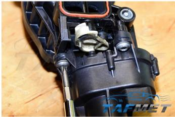
Remove inlet manifold from the engine. Remove 3 bolts which hold the actuator to the manifold. We recommend you wash the manifold using a suitable cleaning fluid.
