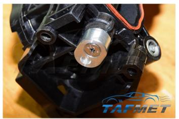
The plug is designed to be a tight fit. A light impact with a hammer may be necessary to push the bung fully into the manifold.
