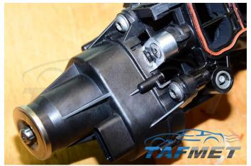
Reinstall the actuator motor. The plastic actuator arm is not required and should be removed. Reinstall the inlet manifold to the engine. There should be no EML and the car should not require reprogramming.
