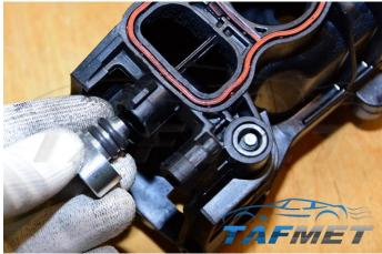
Apply some oil onto the rubber O-rings on the plug. Insert the plug into the hole.
