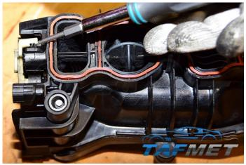
Remove the plastic tie, connecting the axis of the swirl flaps with the actuator motor.
